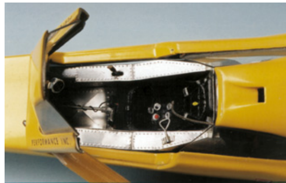
Check out the hand formed aluminum sheeting that was carefully dimpled to suggest rivets. The excellent build quality lead to the survival of this model.
