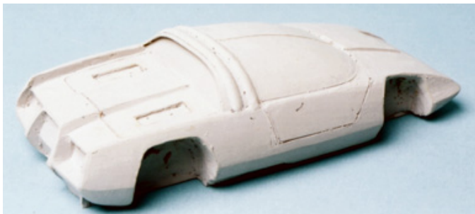
Chuck recreated the original body in clay and then pulled a model and filled it with resin and fiberglass cloth. We have plans to have this body
